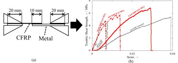
Fig. 1 Schematic drawing of shearing test (a) and tensile shear stress – strain curves at low accumulative probability of the shear strength ( $P_s$ =0.15) of CFRP/Metals (Cu, Al and 18-8) laminated sheets with and without 0.22 MGy-HLEBI (b).
